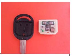
Unscrew small screw at the back of plastic shell. Praise open remote placing your fingernail in the small cut out located at the key shaft end. Separate all parts: top hard shell part with button key pad, part with electronic board and bottom hard shell part.
