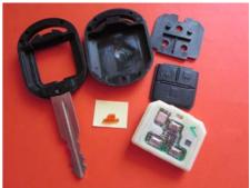
Next remove old key button pad, from the top part of your remote. Button key pad consists of 2 parts (buttons part and plastic support frame) they have to be separated further for your remote to look like the one in the picture above. Just watch for little red plastic light cover that will need to be re fitted later on.
